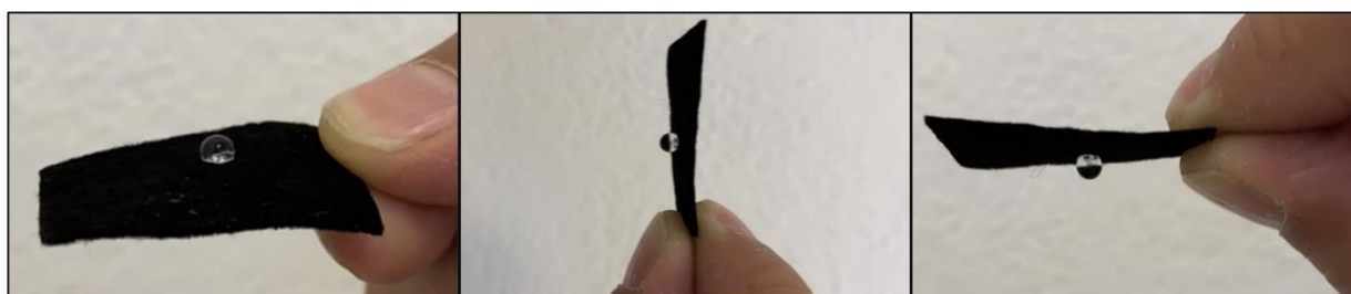
Figure 6. Optical images from three distinct positions of a water droplet on a PET/PPy/ \text{Fe}_3\text{O}_4 composite surface. *The polymerization conditions at [\text{PPy}] = 0.1 \text{ M} and [\text{APS}] = 0.15 \text{ M}
