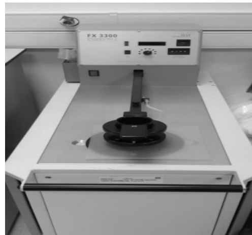
Figure 5. Textest AG - Air Permeability III Fx 3300 Tester
