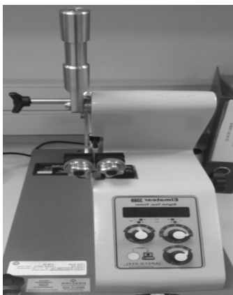
Figure 3. Jeames Heal Elmatear Tear Strength Tester
