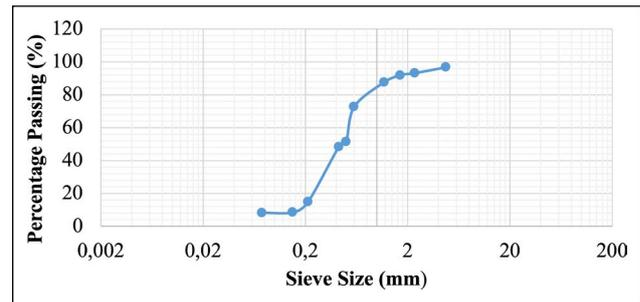
Figure 2. Particle size distribution curve for soil sample.
