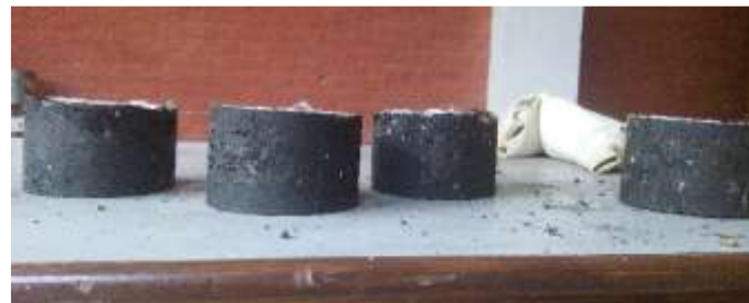
Fig 8. Two specimens on the left containing cement fillers at 6% bitumen content and remaining specimen contains stone dust filler
