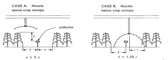
Figure 1. Collector layout for determining the water distribution of lateral move irrigation machines (ASAE, 2012)
