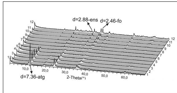
Figure 4- XRD block diagram of sample 6. The numbers 1: Dried, 2:200°C, 3:400 °C, 4:500°C, 5:550°C, 6:600°C, 7:650°C, 8:700°C, 9:800°C, 10:900°C, 11:1000°C, 12:1100°C show the XRD analyses at that temperatures. (atg: antigorite, fo: forsterite, ens:enstatite)
