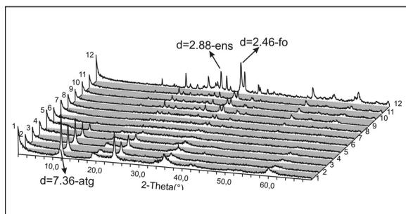
Figure 7-XRD block diagram of sample 29A. The numbers 1: Dried, 2:200°C, 3:400 °C, 4:500°C, 5:550°C, 6:600°C, 7:650°C, 8:700°C, 9:800°C, 10:900°C, 11:1000°C, 12:1100°C show the XRD analyses at that temperatures. (atg: antigorite, fo: forsterite, ens:enstatite)
