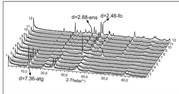
Figure 3- XRD block diagram of sample 1. The numbers 1: Dried, 2:200°C, 3:400 °C, 4:500°C, 5:550°C, 6:600°C, 7:650°C, 8:700°C, 9:800°C, 10:900°C, 11:1000°C, 12:1100°C show the XRD analyses at that temperatures. (atg: antigorite, fo: forsterite, ens:enstatite)
