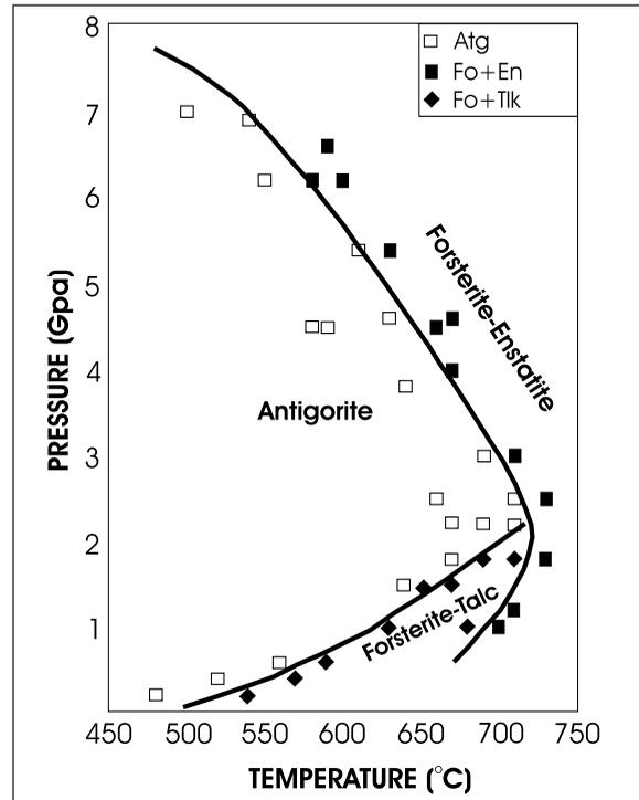
Figure 15- Stability limit of antigorite (Ulmer ve Trommsdorf, 1995)
