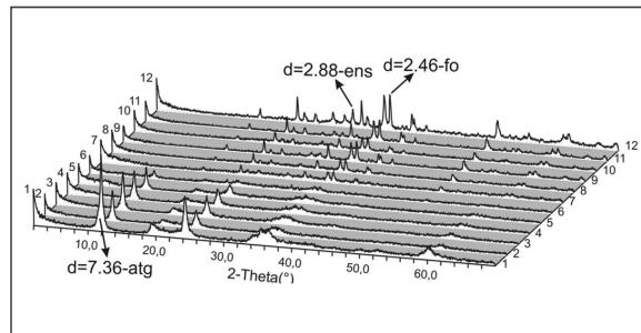
Figure 5- XRD block diagram of sample 11B. The numbers 1: Dried, 2:200°C, 3:400 °C, 4:500°C, 5:550°C, 6:600°C, 7:650°C, 8:700°C, 9:800°C, 10:900°C, 11:1000°C, 12:1100°C show the XRD analyses at that temperatures. (atg: antigorite, fo: forsterite, ens:enstatite)
