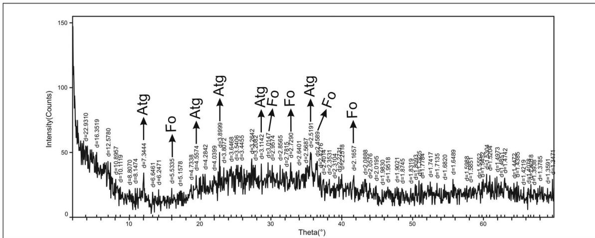
Figure 8- The amorphousization at 600°C (Sample 29A, Atg: antigorite, Fo: Forsterite)
