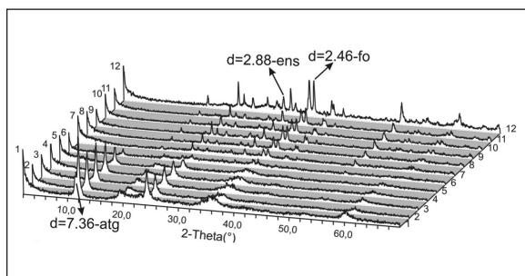
Figure 6-XRD block diagram of sample 11S. The numbers 1: Dried, 2:200°C, 3:400 °C, 4:500°C, 5:550°C, 6:600°C, 7:650°C, 8:700°C, 9:800°C, 10:900°C, 11:1000°C, 12:1100°C show the XRD analyses at that temperatures. (atg: antigorite, fo: forsterite, ens:enstatite)
