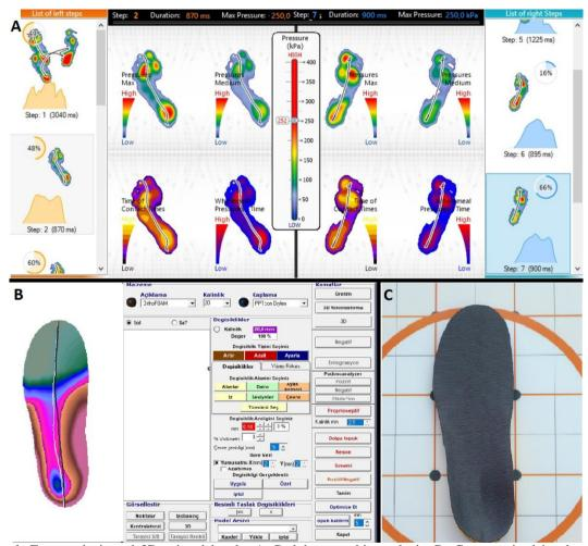
**Figure 1.** Foot analysis and 3D printed insole. A: Pedobarographic analysis, B: Computerized insoles design according to the analysis results, C: Personilized 3D printed insole
