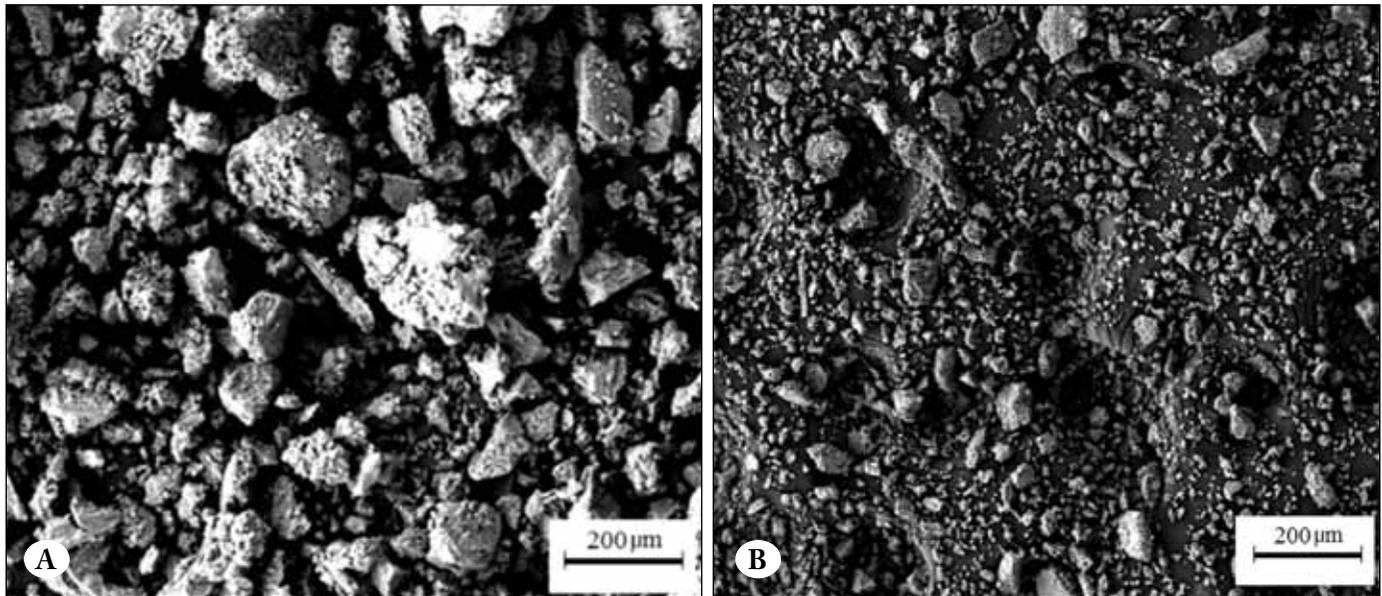
Figure 5. SEM images of the synthesized samples A) NaB(OH)<sub>4</sub>·2H<sub>2</sub>O, B) NaB(OH)<sub>4</sub>
