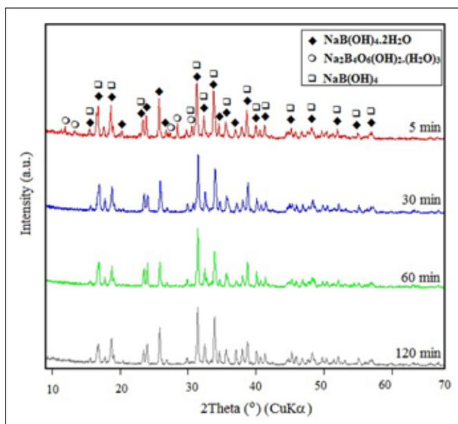
Figure 1. XRD pattern of the samples synthesized by UM.
