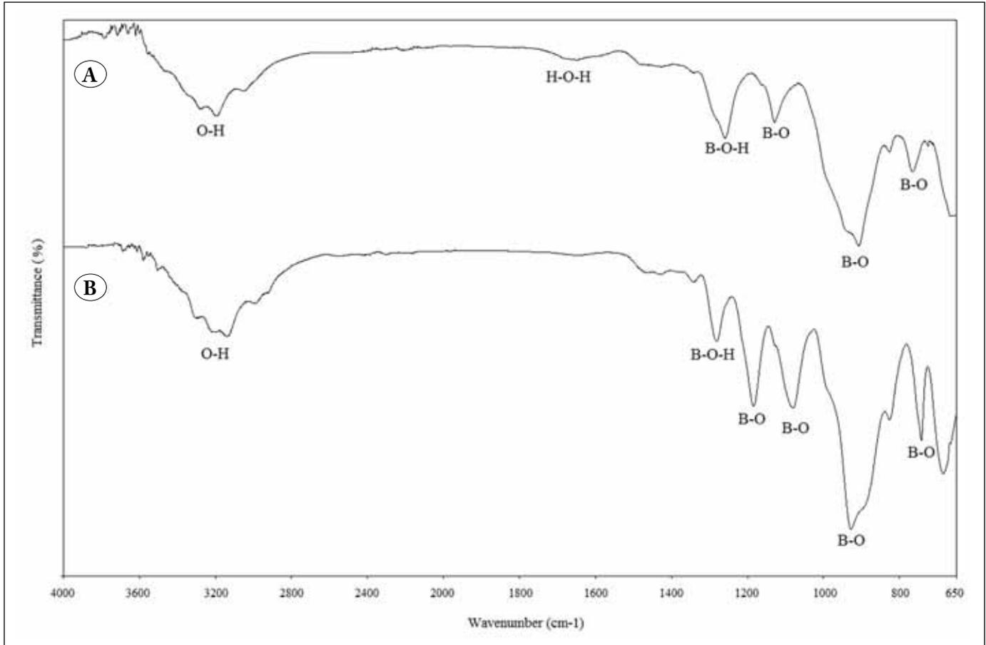
Figure 4. FTIR spectra of the samples synthesized by A) UM, B) CM.
