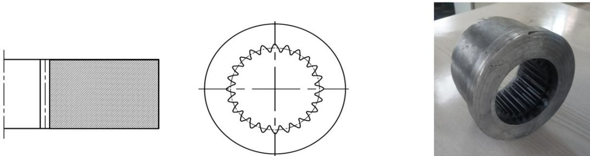
**Figure 3.** The asymmetric gear forging die
