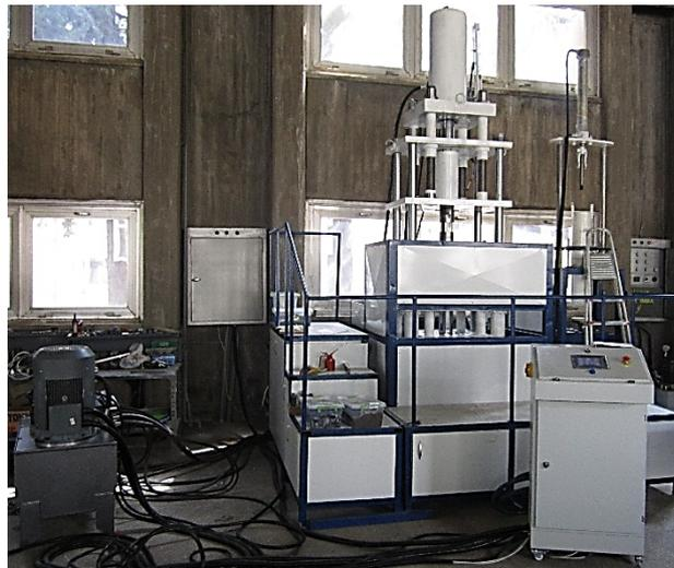
**Figure 1.** Two-way abrasive flow machine
