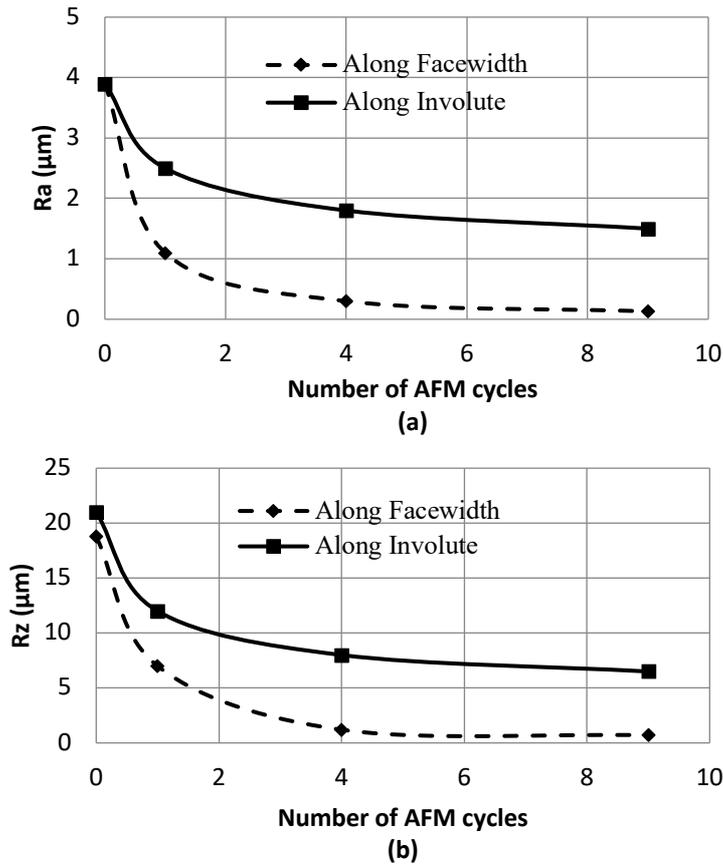
Figure 4. Surface roughness values on gear die tooth a) Ra (μm) and b) Rz (μm)
