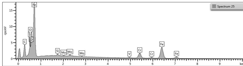
**Figure 2.** EDX Spectrum of the die material
