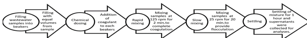
Figure 1. Experimental configuration of coagulation-flocculation process
