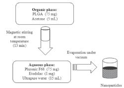
**Figure 3** Nanoprecipitation method used for the preparation of nanoparticles
