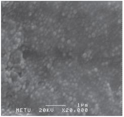
Figure 4 SEM of PLGA nanoparticles
