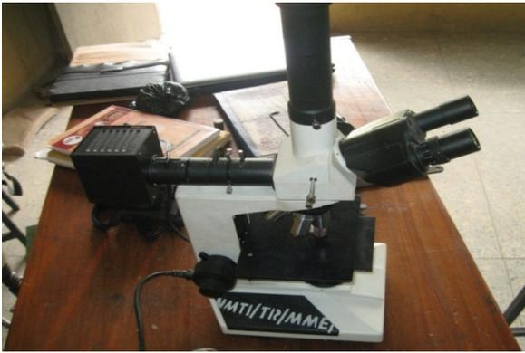
Fig. 1: Optical Metallurgical Microscope
