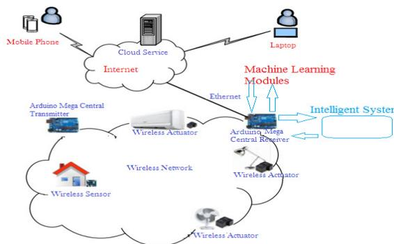
Figure 5 Physical Representation of Smart Home System using wireless Network
