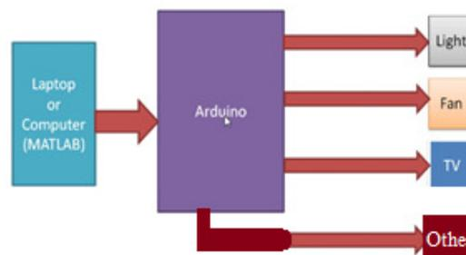
Figure 4 Flow Diagram of smart home appliances
