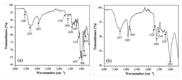
**Figure 4.** The vibrational frequencies and intensities of the bonds present in (a) SPC and (b) SPC/TCH FTIR spectra.
