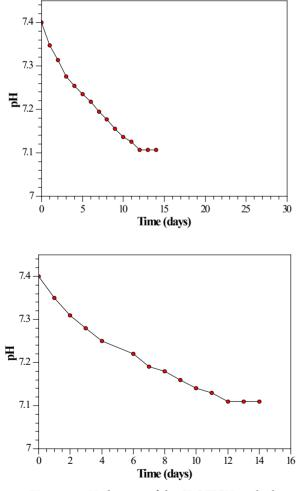
**Figure 6.** pH changes of the SPC/TCH soaked in PBS for 14 days.
