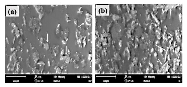
**Figure 2.** SEM micrographs of (a) SPC showing SiO<sub>2</sub> embedded in PHB matrix and (b) SPC/TCH; where SiO<sub>2</sub> and TCH are embedded in the PHB matrix. White arrows show some embedment sites.
