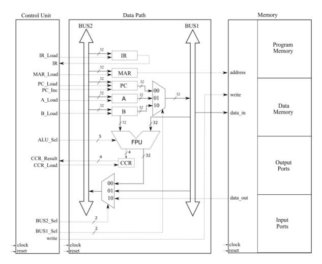
Figure 4. RISC processor micro architecture.
