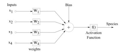
Figure 10. An artificial neural network architecture for Iris classification
