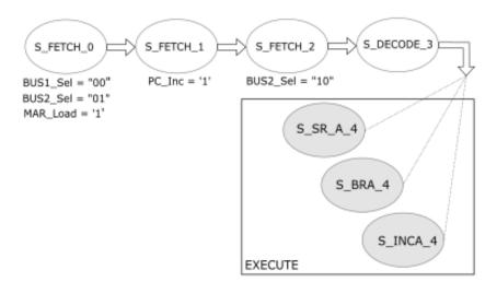
Figure 6. Fetch, Decode and Execute stages
