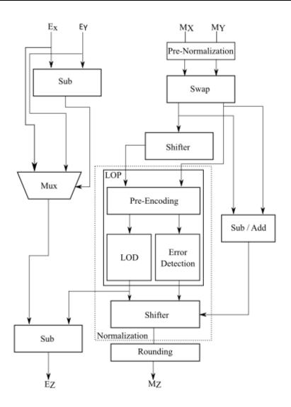
Figure 1. Adder/subtractor micro-architecture
