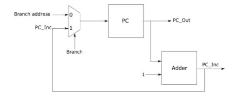
Figure 7. PC register structure
