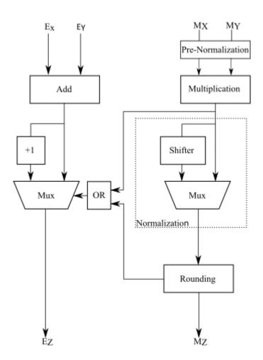
Figure 2. Multiplier micro architecture
