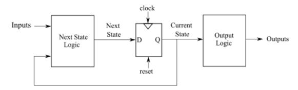
Figure 5. Control unit FSM
