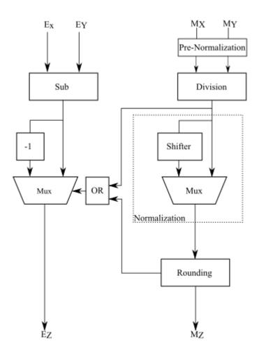
Figure 3. Floating-point divider micro architecture
