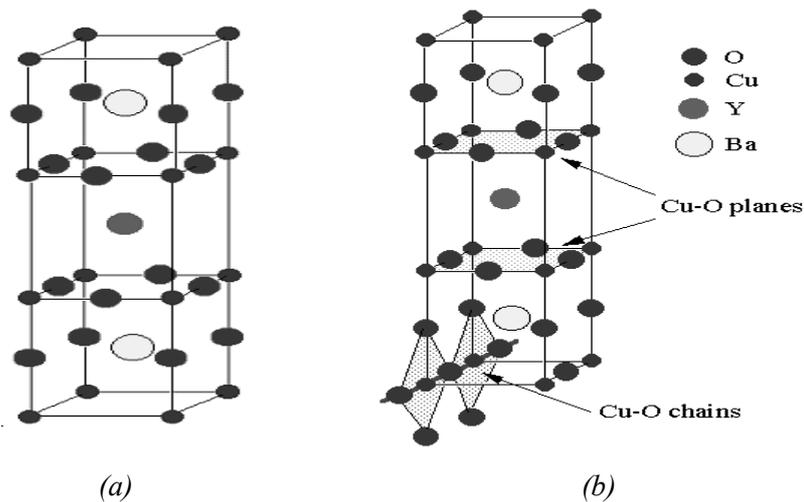
**Figure 1.** (a)  $\text{YBa}_2\text{Cu}_3\text{O}_6$  (a) and  $\text{YBa}_2\text{Cu}_3\text{O}_7$  (b) crystal structures of superconductor compounds
