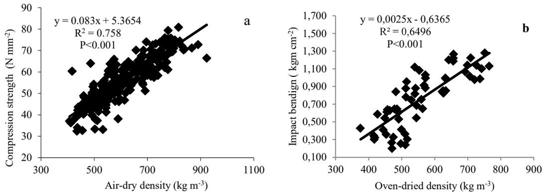
**Figure 2.** Relationships between (a) density and compression strength and (b) and impact bending
