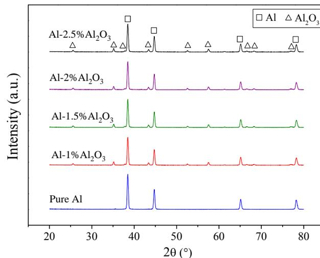
Figure 7. XRD plots of sintered Al-Al<sub>2</sub>O<sub>3</sub> composites and pure Al
