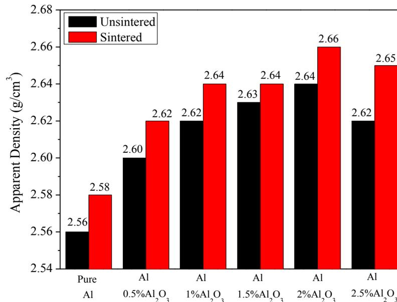
**Figure 4.** The apparent density variation for Al-Al<sub>2</sub>O<sub>3</sub> composites and pure Al
