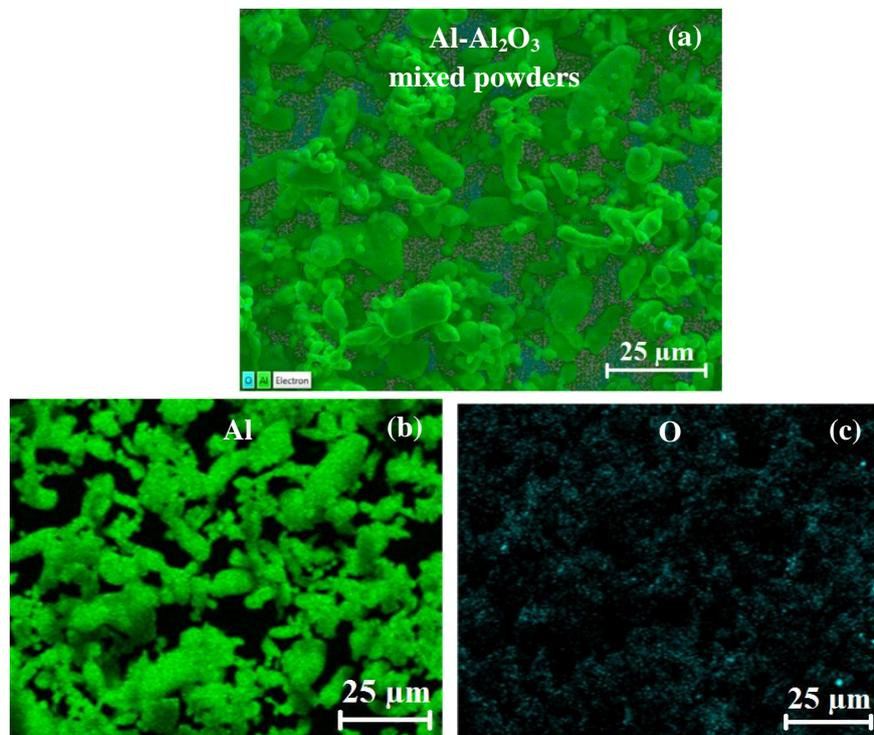
**Figure 3.** SEM-EDX images of Al-2% $\text{Al}_2\text{O}_3$  mixed powders (a), Al (b) and O (c) distribution in mixed powders
