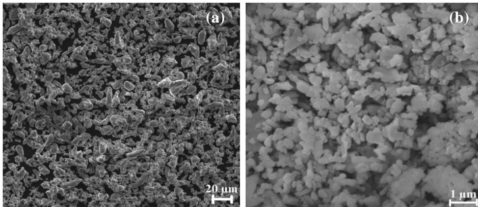
**Figure 2.** SEM images of pure Al (a) and nano alumina ( $\text{Al}_2\text{O}_3$ ) powders (b)
