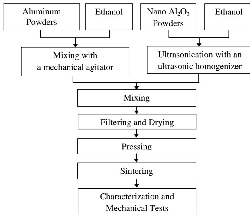
**Figure 1.** Fabrication schemes of Al-Al<sub>2</sub>O<sub>3</sub> composites by powder metallurgy method [15]
