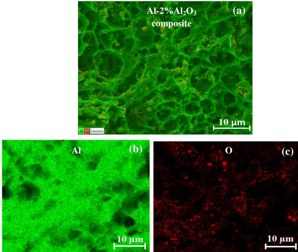
**Figure 9.** SEM-EDX mapping images of Al-2%Al<sub>2</sub>O<sub>3</sub> (a) and Al (b) and O (c) distribution in Al-2%Al<sub>2</sub>O<sub>3</sub> composite
