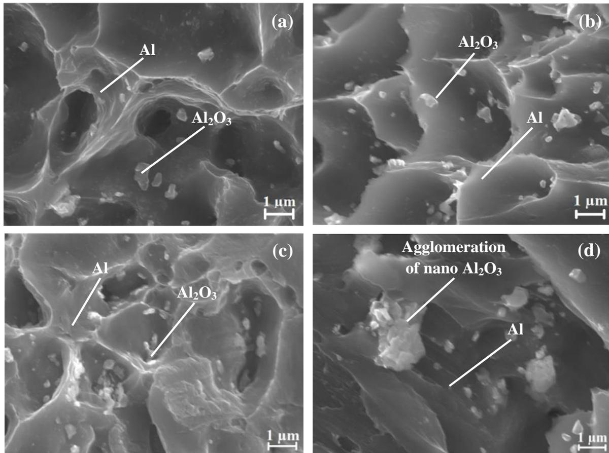
**Figure 8.** SEM images of 1% (a), 1.5% (b), 2% (c), and 2.5% (d)  $\text{Al}_2\text{O}_3$  reinforced Al composites
