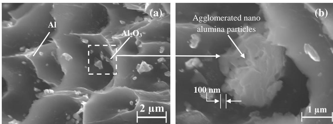
**Figure 10.** The microstructure images of Al-2.5%Al<sub>2</sub>O<sub>3</sub> composite with low (a) and high magnification (b)
