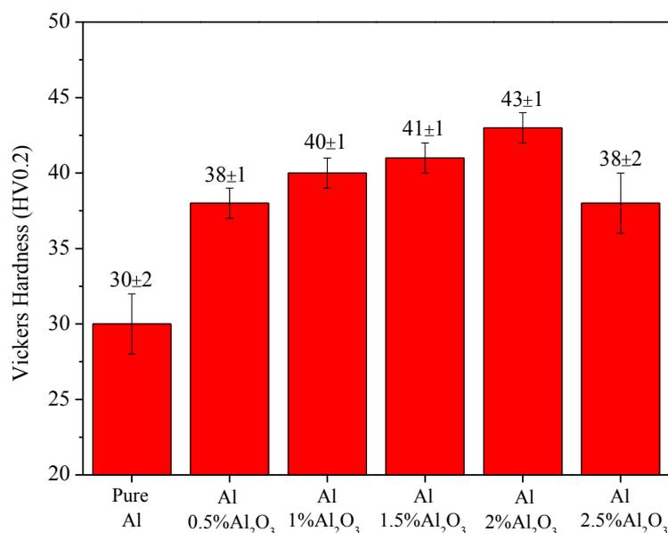
**Figure 5.** The Vickers hardness variation for sintered Al-Al<sub>2</sub>O<sub>3</sub> composites and pure Al
