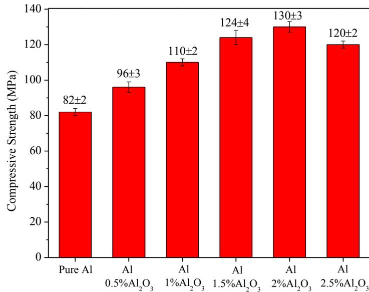
Figure 6. The compressive strength variation for sintered Al-Al<sub>2</sub>O<sub>3</sub> composites and pure Al
