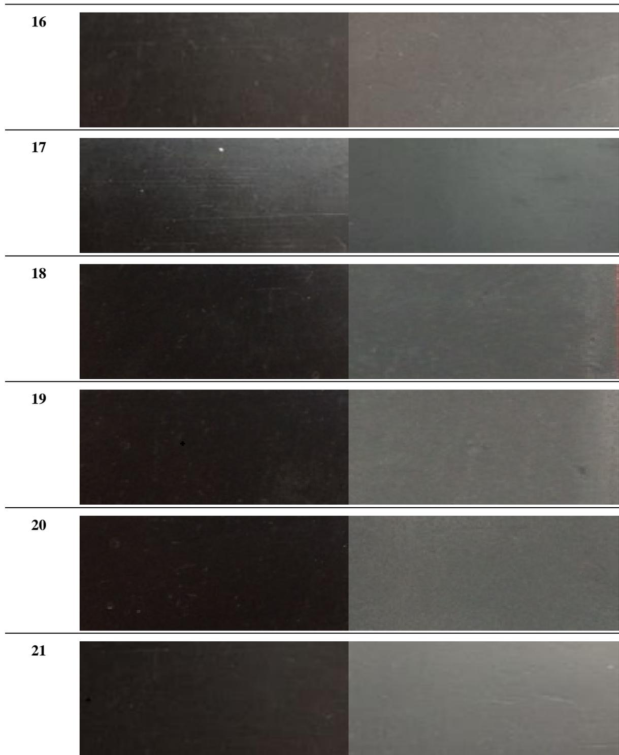
Surface cracks and color changes can be observed on the surfaces after 100 h and 250 h of Florida aging until EPDM plate 14. The surfaces of plates 14 through 21 were more protected against UV-light than those of the others.
