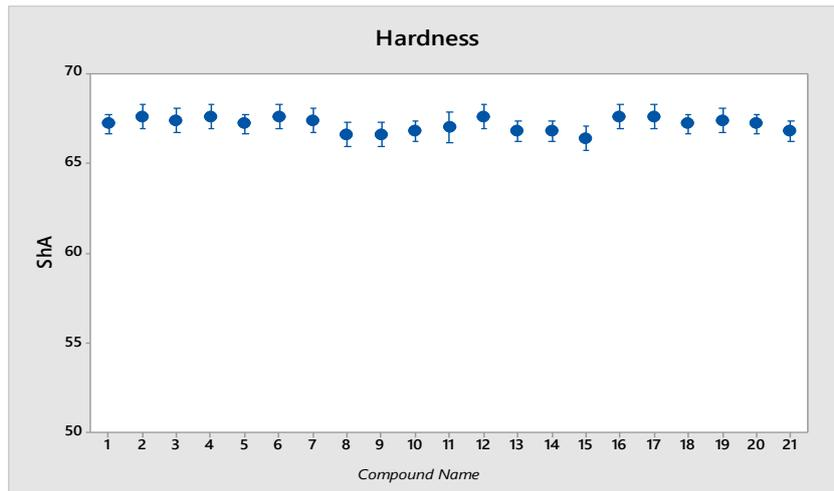
**Figure 5.** UV stabilizers effect on hardness
