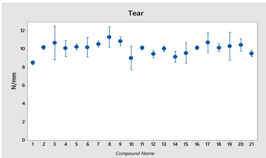
**Figure 3.** UV stabilizers effect on the mechanical properties such as tear strength
