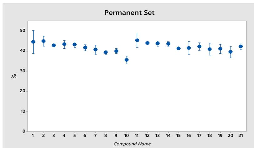
**Figure 6.** UV stabilizers effect on compression behavior
