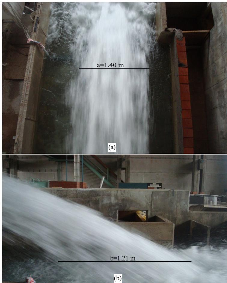
**Figure 7** Lateral (a) and longitudinal (b) dimensions of the dispersed jet for  $Q = 0.22 \text{ m}^3/\text{s}$
