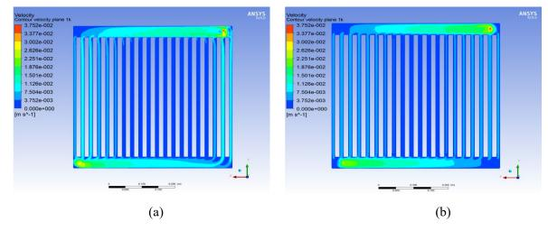
Figure 5. Velocity contours: a. 100% Water fluid, b. 90% Water +10% Propylene glycol fluid
