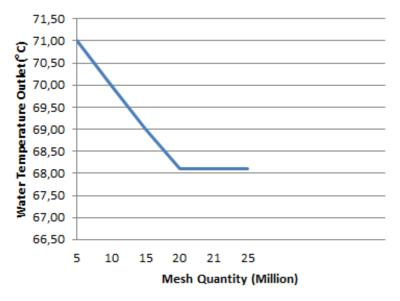
Figure 3. Mesh quantity definition
