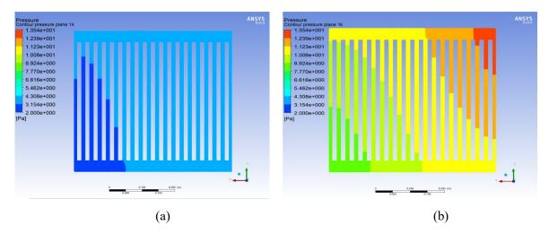
Figure 6. Pressure contours: a. 100% Water fluid, b. 90% Water +10% Propylene glycol fluid
