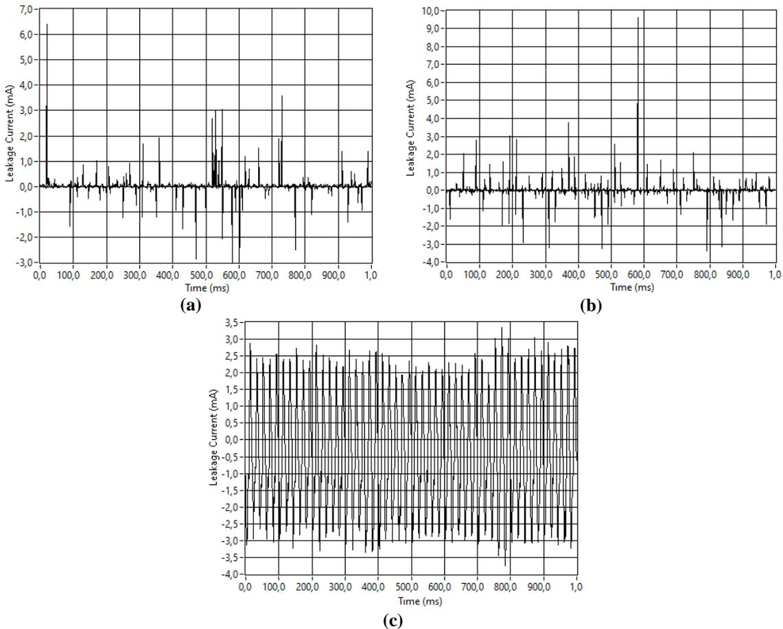
**Figure 7.** For an iced (a) porcelain, (b) glass, (c) silicone insulator with a conductivity of  $4000 \mu\text{S}/\text{cm}$ , the leakage currents obtained under a voltage of 20 kV just before the ice liquefies.
