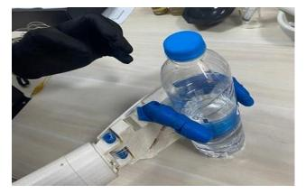
Figure 8. Left skillful hand of the humanoid robot and its control by the glove
