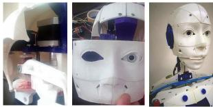
Figure 3. InMoov open source humanoid robot head design
