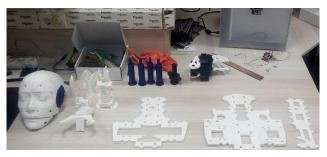
Figure 2. InMoov open source humanoid robotic parts
