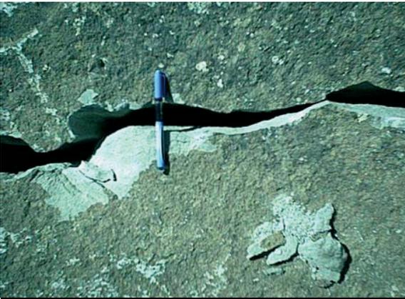
Figure 1. Rock fracture between two neighboring holes due to application of NEEM in a granite mine.
