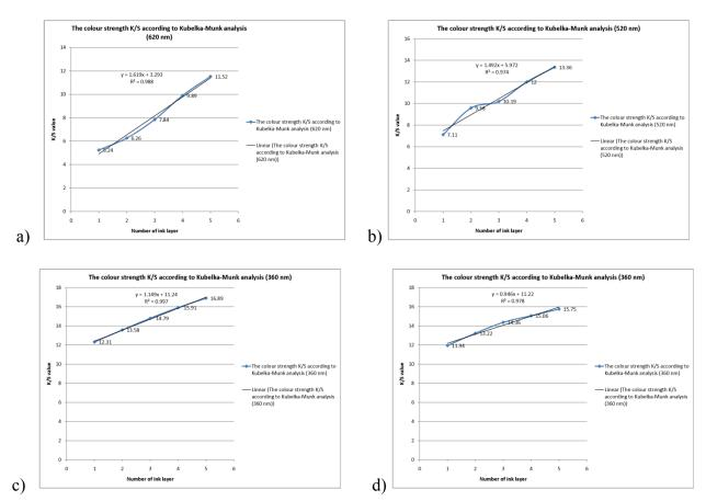
Figure 2. Colour strength K/S according to Kubelka-Munk analysis (material 1) a) cyan, b) magenta, c) yellow, d) black
