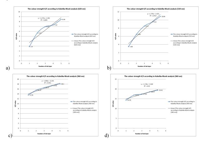
Figure 4. Colour strength K/S according to Kubelka-Munk analysis (material 3) a) cyan, b) magenta, c) yellow, d) black
