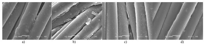
Figure 8. SEM images of material 2 samples, a) before printing, b) after printing, c) after ironing (110 °C), d) after exposure to artificial light and weathering conditions
