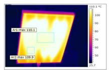
Figure 5. Thermo vision analysis of heat element at 110 °C
