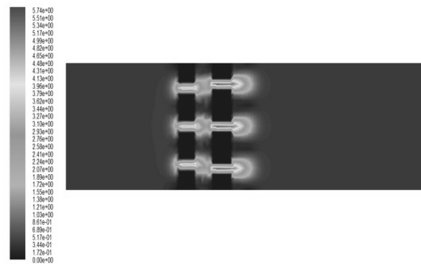
Fig. 10. Visualization of the air transfer through TLS4-6: velocity field (m/s)
