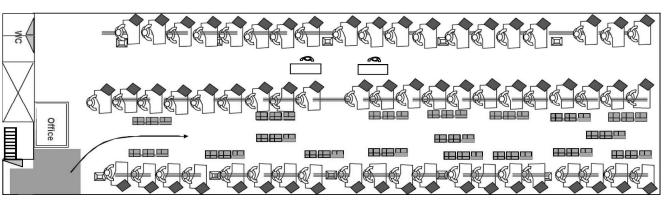
Figure 1. Sample layout of machine in an apparel production company
