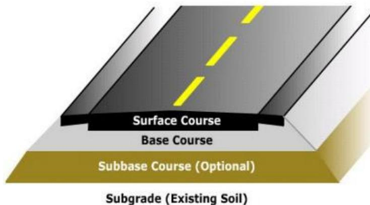
**Figure 3.** A typical flexible pavement section view [23]
