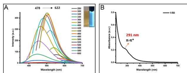
**Figure 1.** Fluorescence spectra of carbon quantum dots at different excitation wavelengths (A) (inset, optic images under daylight (left) and a 365-nm UV light (right)) and UV-vis absorption spectra (B). UV, ultraviolet; vis, visible.
