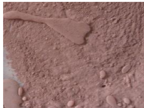
Figure 1. Water droplets escaping out of hydrophobe clay specimen.
