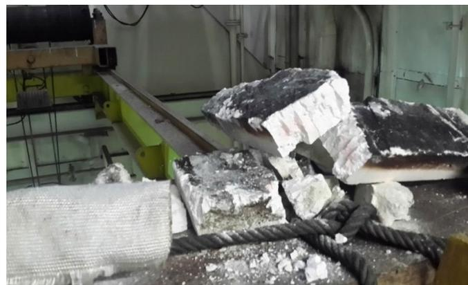
**Figure 6.** The parts which fell off funnel loop
