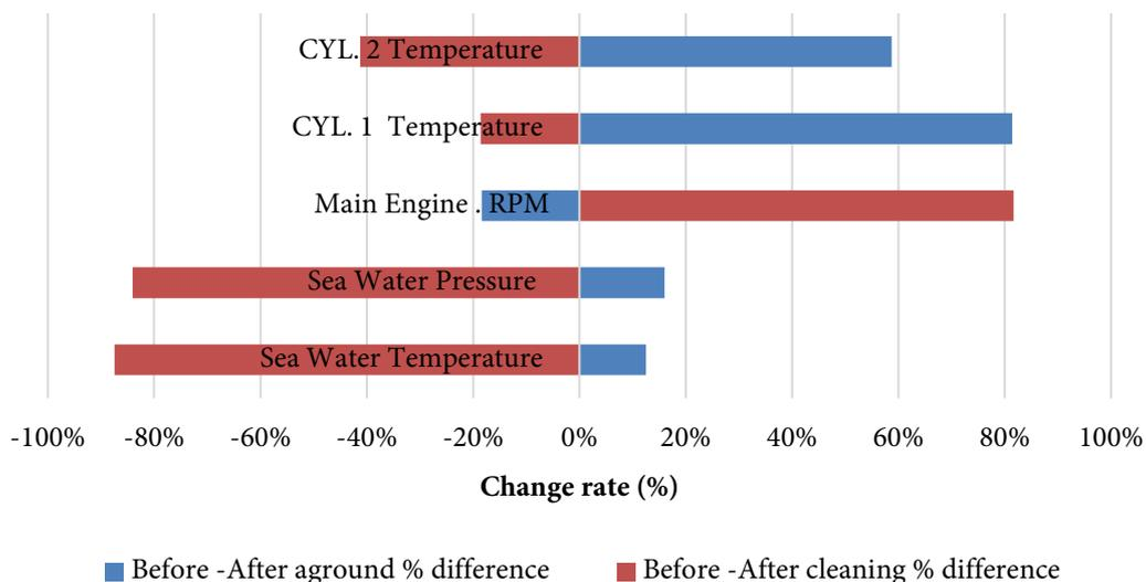
Figure 2. Average changes in the factors affecting the main engine revolution
