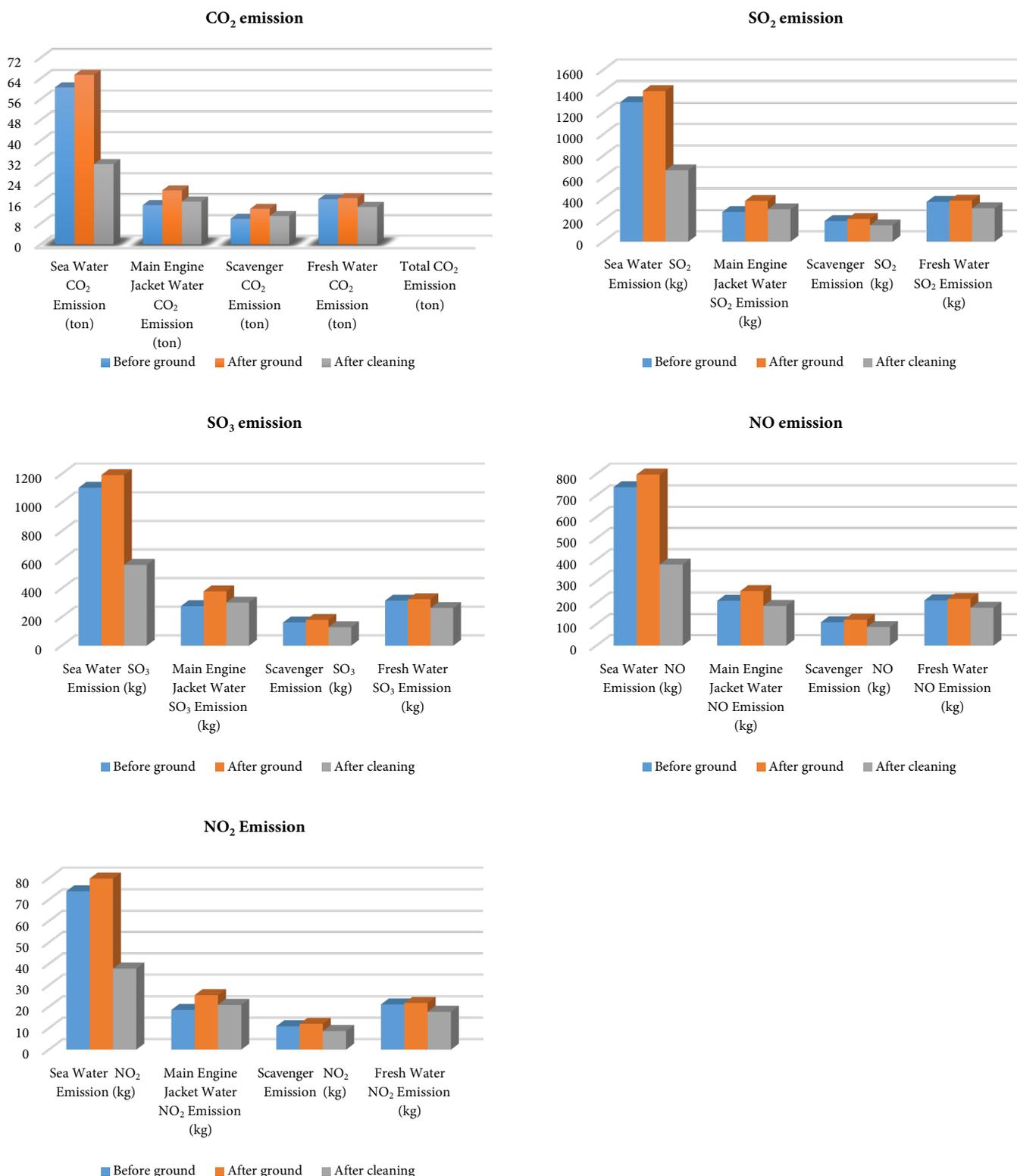
**Figure 7.** Emission change; a) CO<sub>2</sub> emissions, b) SO<sub>2</sub> emissions, c) SO<sub>3</sub> emissions, d) NO emissions, e) NO<sub>2</sub> emissions
