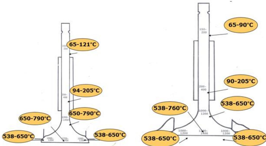
Figure 5. Working temperatures for exhaust (left-side) and intake (right-side) valves.
