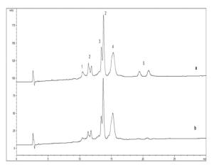
Figure 6. Separation of bovine proteins in raw (a) and pasteurized (b) skimmilk samples diluted with solvent A: solvent B (70:30) mixture by RP-HPLC. Peak identifications are shown;  $1 = \kappa$ -casein,  $2 = \alpha$ -caseins,  $3 = \alpha$ -lactalbumin,  $4 = \beta$ -casein,  $5 = \beta$ -lactoglobulin.
