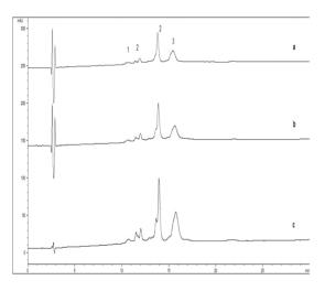
Figure 4. Separation of bovine caseins obtained from pasteurized skimmilk by RP-HPLC using different sample dilution solutions. Chromatograms of casein diluted with phosphate buffer (a), diluted with phosphate buffer contained 0.1 % trifluoroacetic acid (b), diluted with solvent A: solvent B (70:30) mixture (c). Peak identifications are shown;  $1 = \kappa$ -casein,  $2 = \alpha$ -caseins,  $3 = \beta$ -casein.
