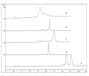
Figure 5. Separation of purified bovine milk protein standards by RP-HPLC. (a):  $\kappa$ -casein, (b):  $\alpha$ -caseins, (c):  $\beta$ -casein, (d):  $\alpha$ -lactalbumin, (e):  $\beta$ -lactoglobulin.
