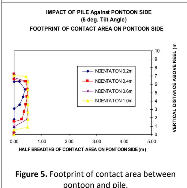
Figure 5. Footprint of contact area between pontoon and pile.
