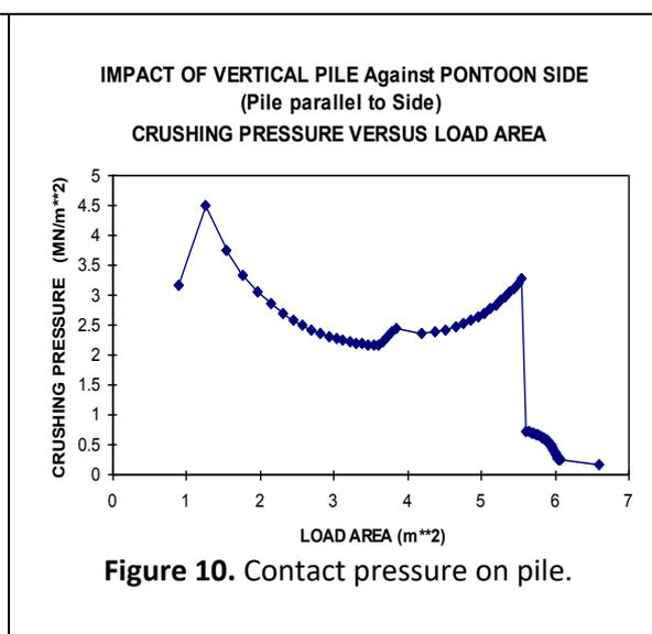
The plastic deformation resistance of the considered pontoon structure will vary with the striking angle between the side of the pontoon and the struck vertical pile (angle in the vertical plane). The highest loads will occur when the pile and the pontoon side are parallel at the impact, i.e. contact over the total height of the pontoon side. On the other hand the average contact pressure on the pile when penetrating into the pontoon side will not vary significantly with the striking angle.
