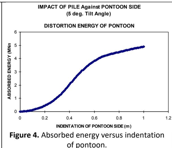
Figure 4. Absorbed energy versus indentation of pontoon.
