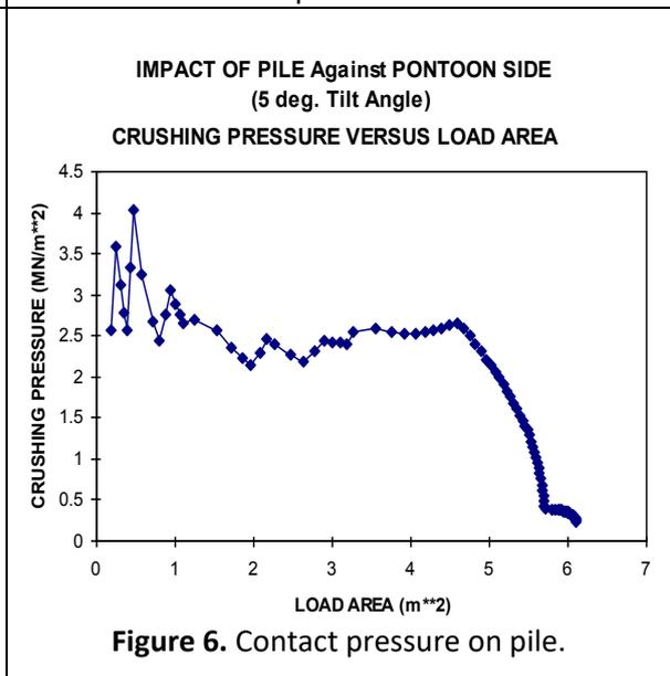
Figure 6. Contact pressure on pile.
