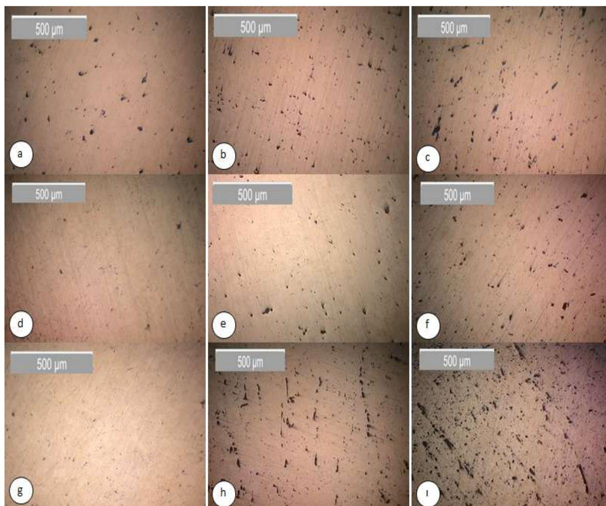
**Figure 4.** Microstructural images of the pure aluminum sample manufactured using P/M technique at different sintering temperatures and for different durations a) 500°C / 45 min., b) 500°C / 60 min., c) 500°C / 75 min., d) 550°C / 45 min., e) 550°C / 60 min., f) 550°C / 75 min., g) 600°C / 45 min., h) 600°C / 60 min., i) 600°C / 75 min.
