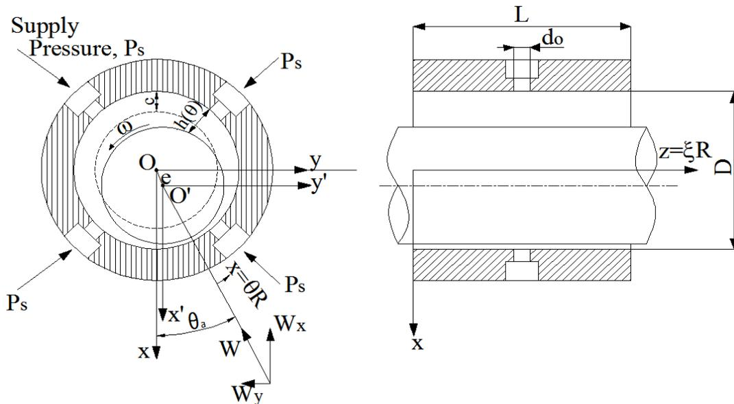
Figure 1. A hydrostatic journal bearing [28]
