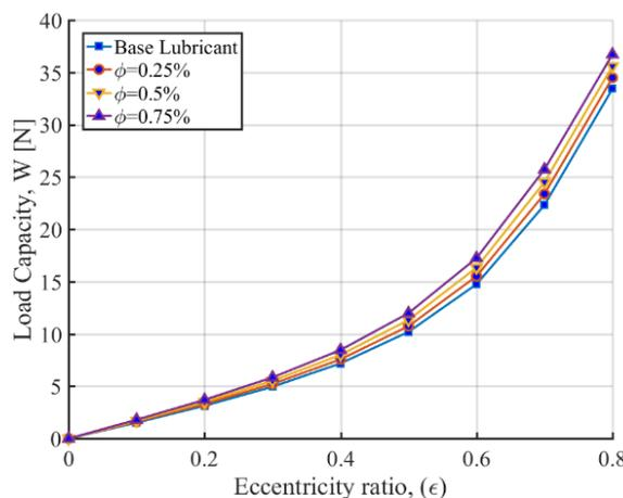
Fig. 4 Variations of the load capacity in regard to the eccentricity ratio for different volumetric ratios of the nanoparticle additive
