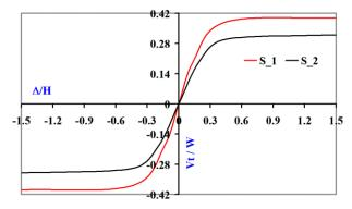
Figure 2. Pushover curves of model buildings e-ISSN: 2148-2683
