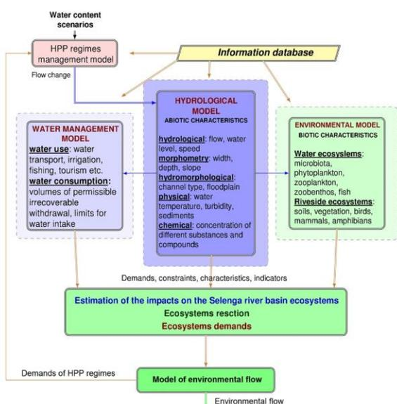
**Figure 3.** The system of models” flow-environment” of the Selenga river.
