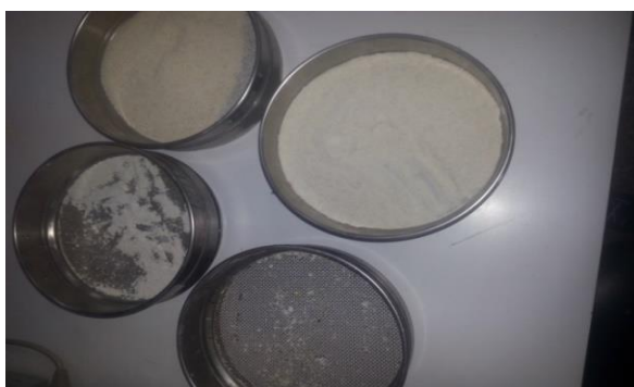
Figure 8. Picture during separation on different sieve sizes of sample flour.
