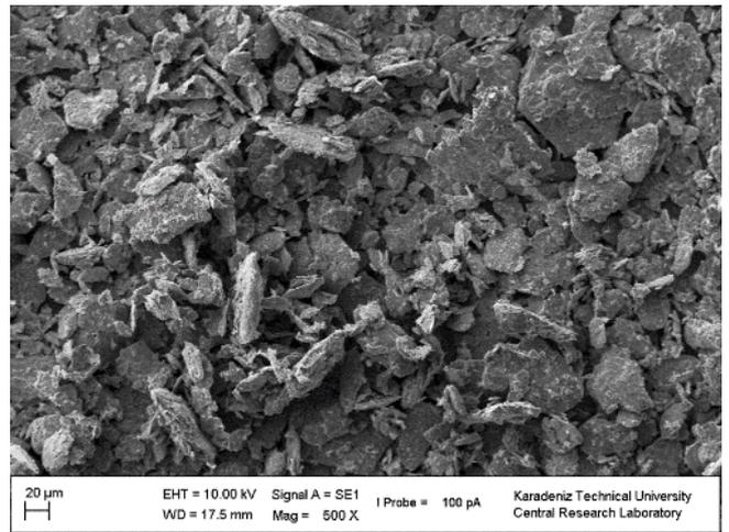
**Figure 3.** SEM morphologies of the MoS<sub>2</sub> nanoparticles
