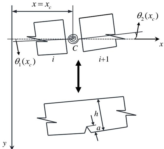
**Figure 2.** Cracked section represented by massless rotational spring.
