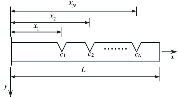
**Figure 1.** A cantilever beam with multiple cracks
