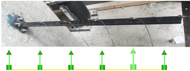
Figure 4. Laboratory model and accelerometer locations.
