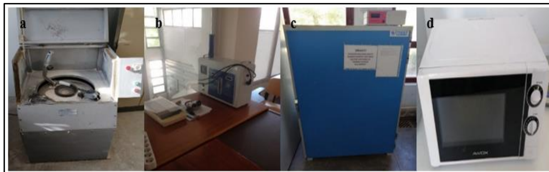
Figure 1. The photos of (a) ringed mill, (b) blaine device, (c) oven and (d) household microwave oven Unit weight (UW) of the aggregates were calculated according to TS EN 1097-6 [19]. Fracture load of aggregates were determined by one point loading device using apparatus given in Fig. 2 to spread the load uniformly. One point loading device was preferred for precise measurement of the little crushing loads. All the reported results are the means of three samples. The crushing strength ( \sigma , kg/cm 2 ) for spherical aggregates are calculated by the equation 1 where: P: fracture load (kN), and X: the distance between loading points (mm) [20, 21]. SEM-EDX analyses on core and shell of the aggregates were conducted.
