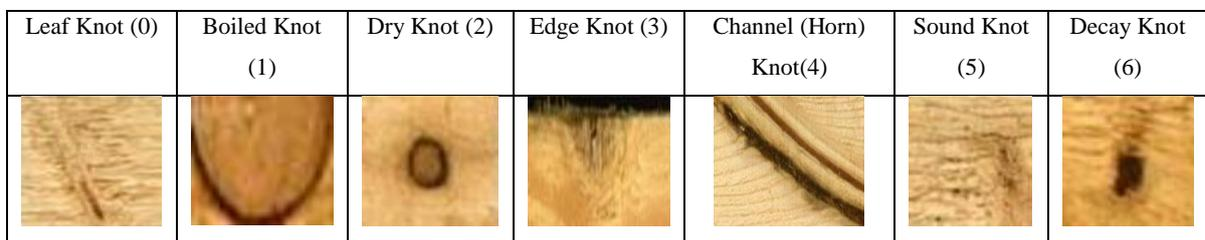
Figure 2: Example of different type knots in wood
