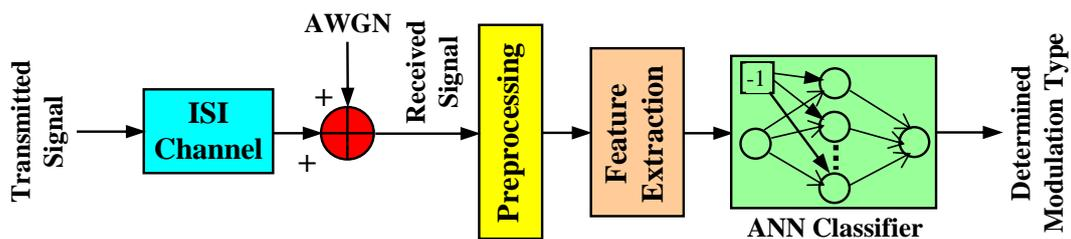
Figure 4. The block diagram of ANN based modulation recognizer in AWGN and frequency selective Rayleigh fading channel.
