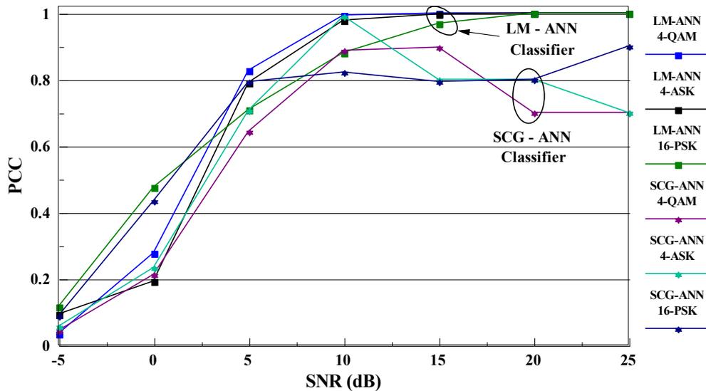
Figure 3. The performances of correct classification of SCG-ANN and LM-ANN recognizers in AWGN channel.
