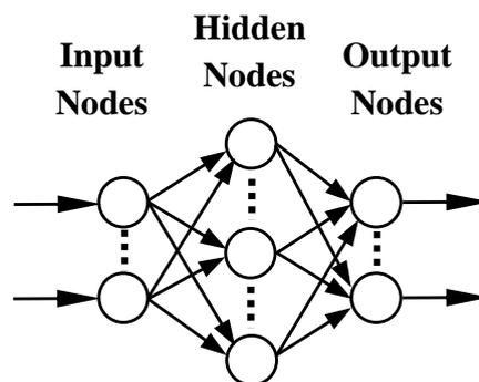
**Figure 2.** A three-layered feedforward neural network structure.
