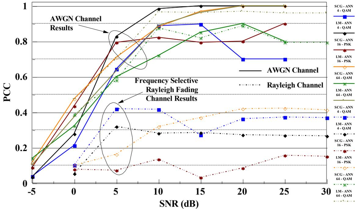
Figure 5. The performances of correct classification of SCG-ANN and LM-ANN recognizers in AWGN channel and frequency selective Rayleigh fading channels.
