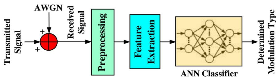
**Figure 1.** The block diagram of ANNs based modulation recognizer in AWGN channel.
