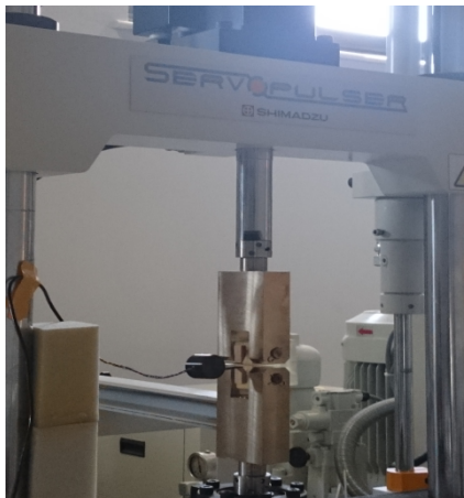
Figure 2. Fracture test setup
