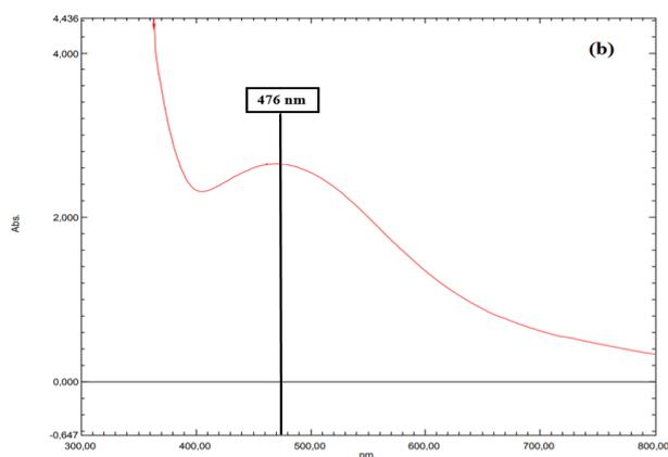
**Figure 2.** Maximum absorbance value of AgNPs synthesized by *Rumex acetosella* L. plant in UV-vis spectroscopy
