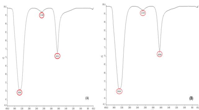
**Figure 3.** Functional groups involved in reduction by FT-IR analysis: a) FT-IR spectrum of *Rumex acetosella* L. plant extract, b) FT-IR spectrum of synthesized AgNPs
