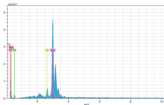
**Figure 6.** Elemental composition of AgNPs synthesized by *Rumex acetosella* L. plant by EDX
