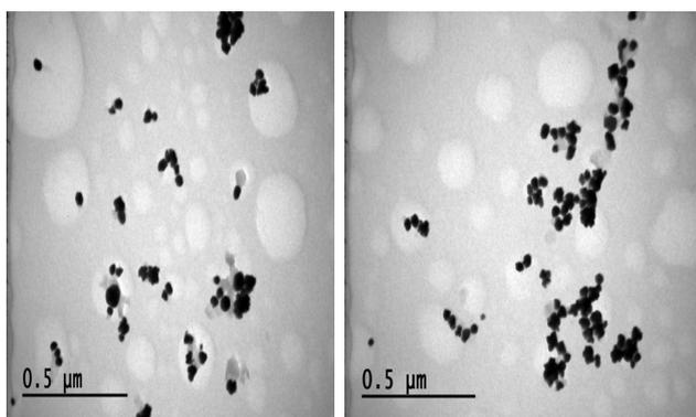
**Figure 7.** TEM images of AgNPs synthesized by *Rumex acetosella* L. plant
