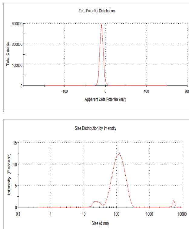
**Figure 8.** a: Zeta potential plot of AgNPs synthesized by *Rumex acetosella* L. plant b: Zeta size plot of AgNPs synthesized by *Rumex acetosella* L. plant
