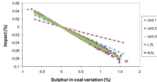
Figure 5: Sulphur in coal increment and its impact on boiler efficiency.
