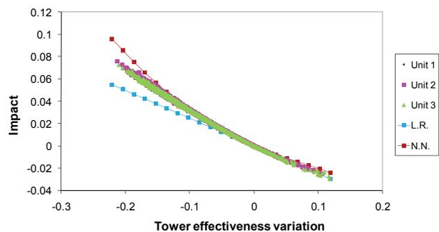
Figure 6: Cooling tower effectiveness increment and its impact on cycle heat rate.
