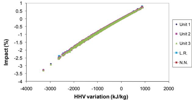
Figure 4: Coal HHV increment and its impact on boiler efficiency.
