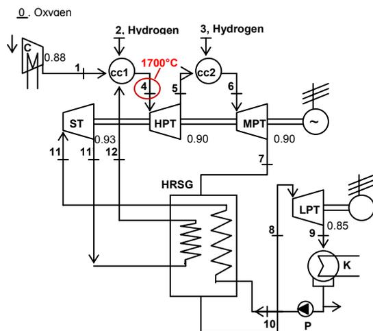
Figure 2. Plant layout of Cycle n°2.
