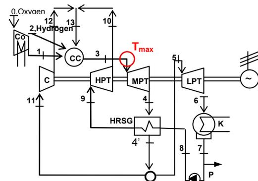
Figure 3. Plant layout of the ZECOTECH® cycle.
