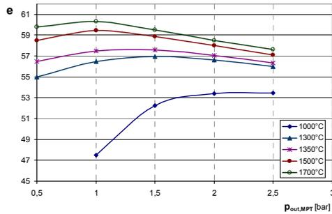
Figure 4. Exergetic efficiency as function of  $P_{out,MPT}$  (Cycle n°3).
