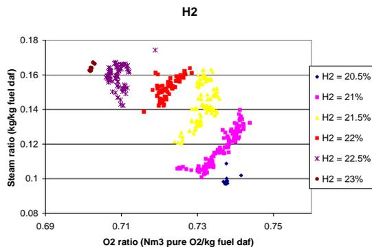
Figure 7. H<sub>2</sub> operations map using ratio transformation and average fuel composition.
