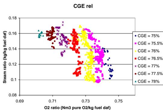
Figure 8. Relative CGE operations map using ratio transformation and average fuel composition.
