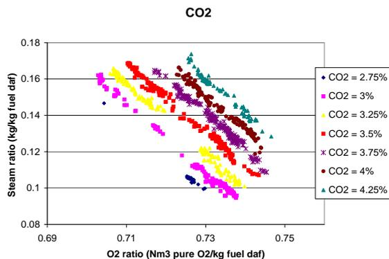
Figure 6. CO<sub>2</sub> operations map using ratio transformation and average fuel composition.
