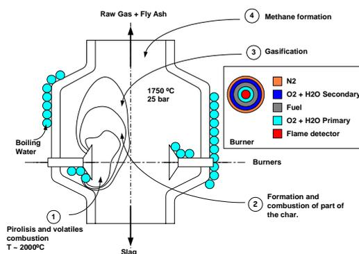
Figure 1. Reaction chamber schematic. Source: Elcogas.
