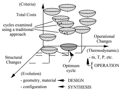
Figure 1. The structural (synthesis-design) and operational (synthesis-operation) space of energy systems (von Spakovsky, 1998).
