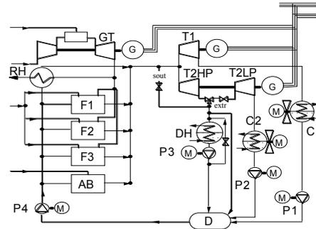
Figure 2. Superconfiguration for the waste incineration cogeneration plant with a gas turbine topping cycle.
